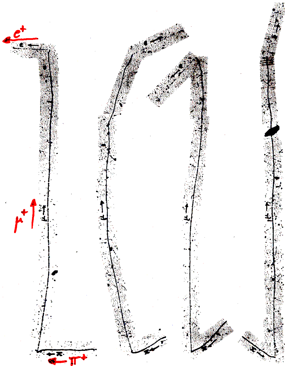
Fig. 1.3 Examples of the decay sequence \pi^+ \rightarrow \mu^+ \rightarrow e^+ in G5 emulsion exposed at Pic du Midi. The constancy of range ( \approx 600 \mu\text{m} ) of the muon implies two-body decay at rest of the pion: \pi^+ \rightarrow \mu^+ + \nu_\mu . The first examples of pion decay were observed by Lattes, Muirhead, Occhialini, and Powell in 1947. The electron emitted in muon decay, \mu^+ \rightarrow e^+ + \nu_e + \bar{\nu}_\mu , was not served in the early experiments employing less sensitive emulsions. (Photograph courtesy University of Bristol).
