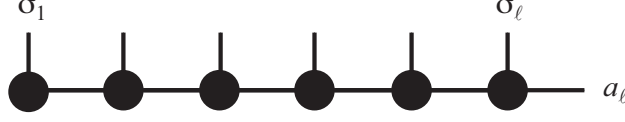
Figure 11: Graphical representation of the recursive construction of a state |a_\ell\rangle by contraction (multiplication) of A -matrices. Contractions run over all connected legs.
