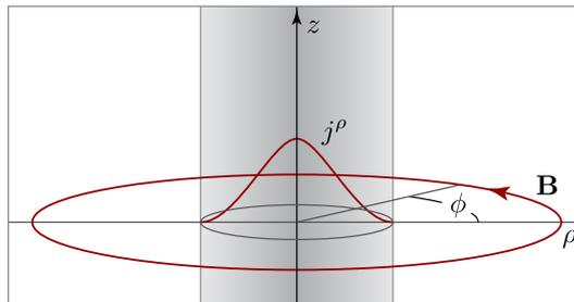
Figure V16: Current distribution and magnetic field of an infinite cylindrical wire (shaded).
