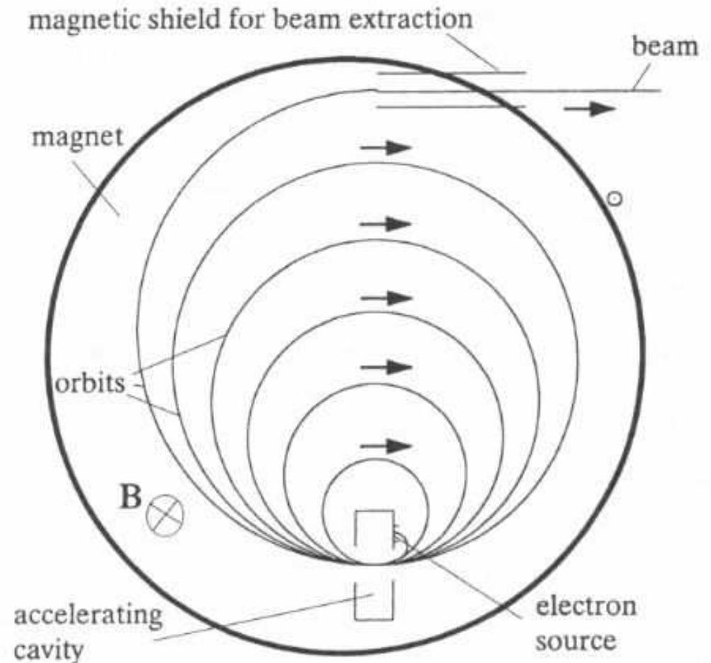
**Fig. 3.2.** The principle of a microtron accelerator (schematic)
