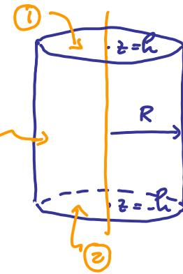
$$\int dV \vec{\nabla} \cdot \vec{v} = ? \quad \vec{\nabla} \cdot \vec{v} = \frac{1}{\rho} \partial_\rho (\rho v_\rho) + \frac{1}{\rho} \partial_\varphi v_\varphi + \partial_z v_z \quad \text{F55}$$
