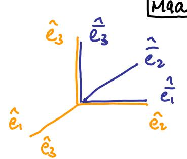
Rotation um  $90^\circ$  um y-Achse:  $D^y(90^\circ)_{jm} = \hat{e}_j \cdot \hat{e}_m = \begin{pmatrix} 0 & 0 & -1 \\ 0 & 1 & 0 \\ 1 & 0 & 0 \end{pmatrix}$  (2)
