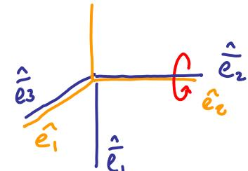
Rotation um  $90^\circ$  um z-Achse:  $D^x(90^\circ)_{jm} = \hat{e}_j \cdot \hat{e}_m = \begin{pmatrix} 1 & 0 & 0 \\ 0 & 0 & 1 \\ 0 & -1 & 0 \end{pmatrix}$  (3)
