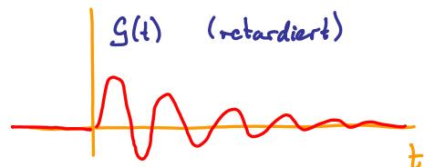
$$G(t) = \Theta(t) \frac{\sin \Omega t}{\Omega} e^{-\gamma t}, \quad \text{mit } \Omega = \sqrt{\omega_0^2 - \gamma^2} \quad (2)$$
