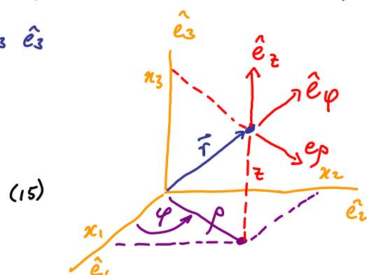
$$(\delta \vec{r})_\rho = \frac{\partial \vec{r}}{\partial \rho} = (\cos \varphi, \sin \varphi, 0), \quad b_\rho = 1 \quad (16a)$$
