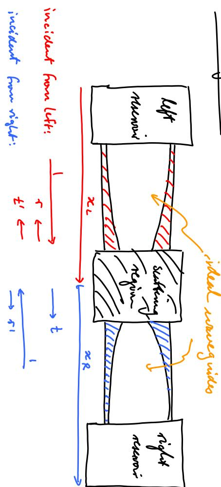
Wavefunctions in left/right waveguides can be described in terms of plane waves.
