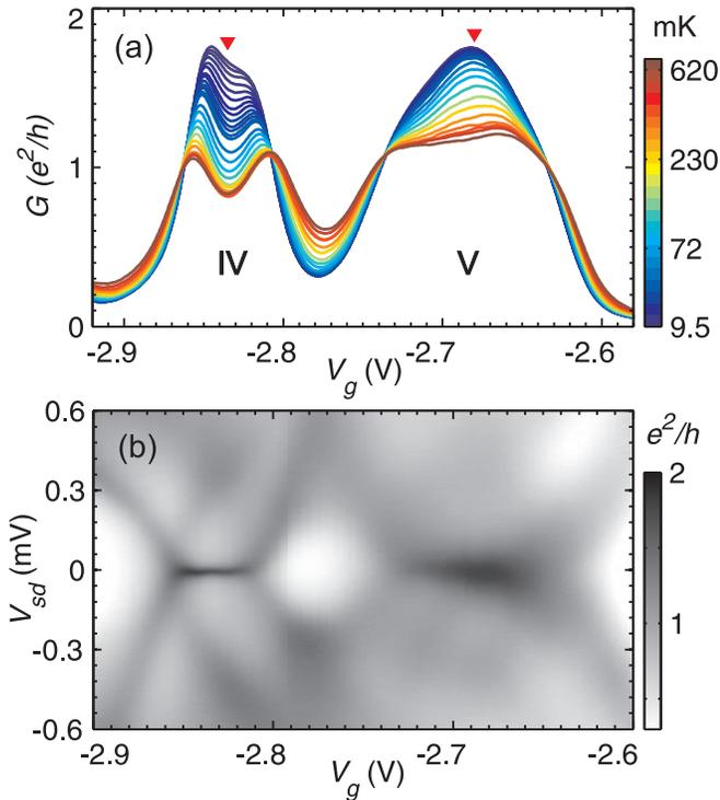
FIG. 3. (a) The detailed measurement of the conductance temperature dependence shown in Fig. 1(a), Valleys IV and V. The red triangles mark two values of  $V_g = -2.835$  V and  $V_g = -2.680$  V for which the conductance as a function of  $V_{sd}$  is plotted in Fig. 4(a) and Fig. 4(b), respectively. (b) The gray-scale conductance plot in the  $V_g - V_{sd}$  plane was measured in the same range of  $V_g$  as in (a), at temperature  $T = 10$  mK.
