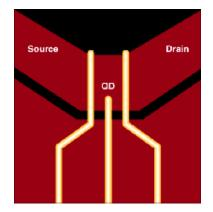
**Experimental realization of a quantum dot (QD).** A QD is a small puddle of charge containing a well-defined number of electrons and is typically fabricated by putting metallic gates (yellow) on a semiconductor region that behaves as a two-dimensional electron gas (red).
