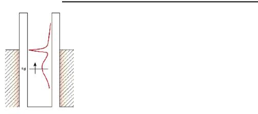
**Effective screening.** Energy diagram for a QD whose density of states (dashed line) has a broad single-particle resonance at the energy of the local level, e<sub>d</sub>, and a sharp Kondo resonance at the chemical potential of the leads.
