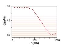
**Toward the unitary limit.** Temperature dependence of the height of the peak in G(V), which saturates near the unitarity limit of  $2e^2/h$  for van der Wiel *et al.*'s QD.
