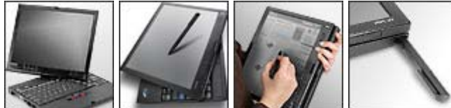
Figure 1: A tablet PC is a regular laptop, but additionally equipped with a special handheld digitizer pen and a screen that can be swivelled 180 degrees and folded screen-side up to serve as electronic notepad for freehand writing. (Shown here: a ThinkPad X41 Tablet PC; I currently use an ACER TravelMate C300). Under Microsoft Windows, it allows freehand writing in several types of documents, including Word, Powerpoint, Windows-Journal (ideal for lecturing) and Adobe-products. (The digitizer pen does not work under Linux.)
